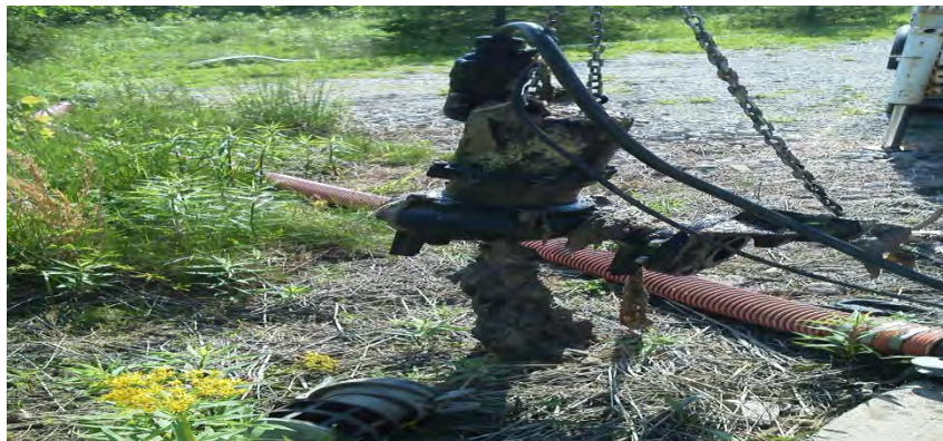
The pump shown from the Rolling Acres lift station was destroyed by the "flushable and disposable" wipes seen hanging from the impeller.
